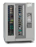
The RoboCrib® LX2000 has been designed to provide secure access for up to 2574 SKUs (unique items). The variety of available bin sizes makes managing both small and large items a reality (carbide inserts, drill bits, spray cans, tape, safety glasses, air tools, welding tips, solder, welding tanks and more!).
